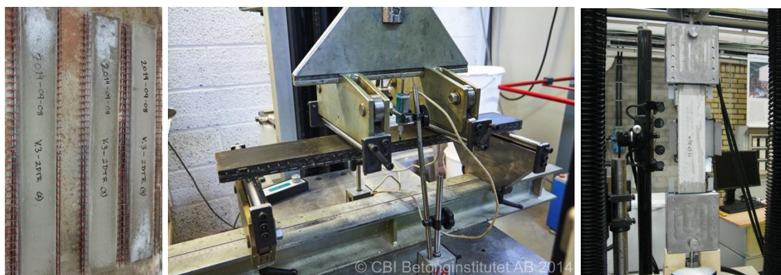
Figure 2 – Panels with carbon fiber grids for bending and tensile tests. Set-up of the 4-point bending test (left) and for the tensile test on panels (right).
